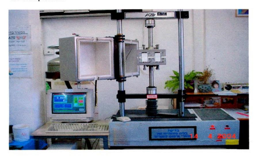
Test specimen in tension of 3.0 mm after 5,000 additional cycles
